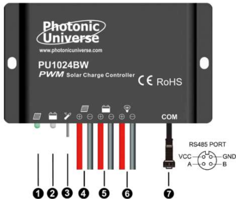
Figure 2: 10A waterproof solar charge controller features
