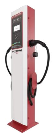
The Hydra Genesis dual-output models require a 400v three-phase electrical supply, which can be found in larger industrial premises and office blocks, which is sufficient to power the Genesis to deliver dual 7kW, 22kW or 43kW charging power (for vehicles which can accommodate the higher AC input).
