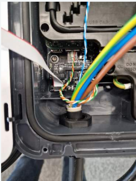
Figure 13: Smart LUX™ Data Cable Routing
