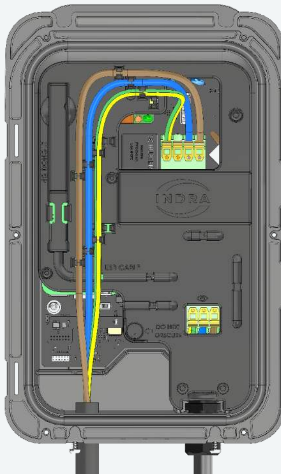
Figure 6: Smart LUX™ Mains Cable Routing
