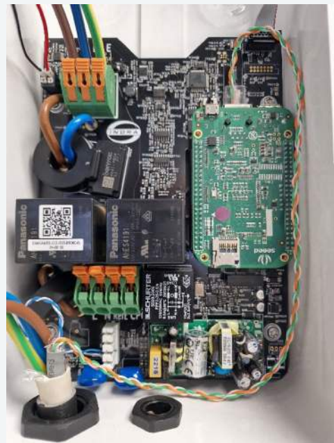
Figure 14: Smart PRO Data Cable Routing
