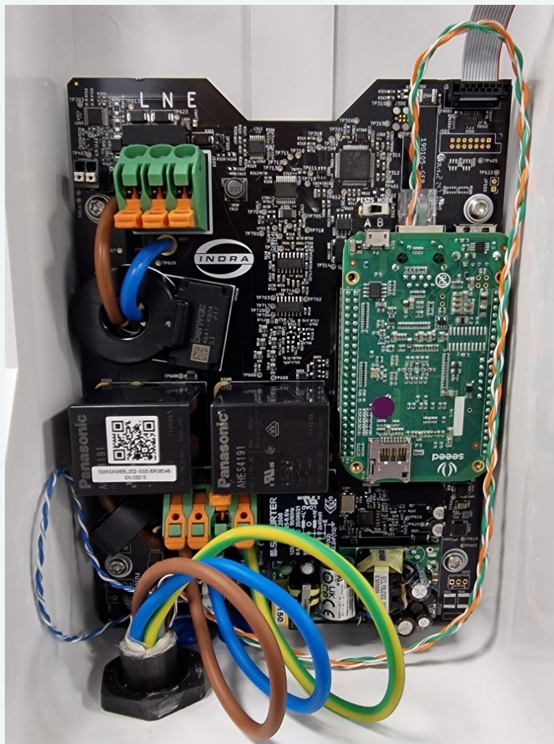
Figure 7: Smart PRO Mains Cable Routing
