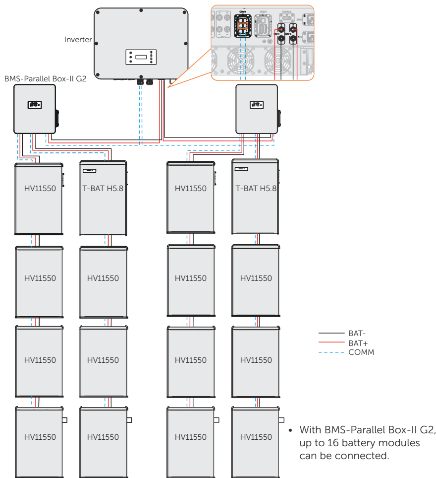
Figure 8-25 Battery connection with BMS-Parallel Box-II G2
