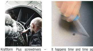
It happens time and time again that the tip slips out of the screw head when screwdriving, sometimes damaging valuable surfaces or even causing injury. The tips of the Wera Lasertip screwdrivers are microscopically roughened by means of a laser. This rough surface literally "bites" itself firmly into the screw head. Slipping out becomes a thing of the past.
